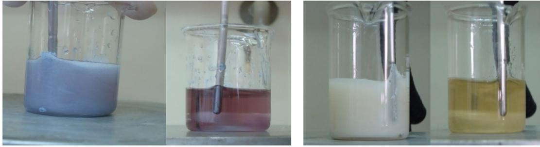
**Figure 6** Neodymium (left) and Lanthanum (right) oxide dissolving in neat EmimHSO<sub>4</sub> at elevated temperatures. The solution becomes clear in less than 5 minutes at 210 °C.
